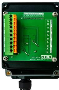
NGS-100 is a NMEA selector switch to provide 1 outputs from 4 inputs. It has a built-in selector PCB for easy connection.
